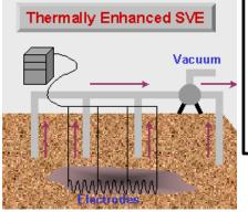
In situ desorbing PFAS from soil particles into gas phase by heating, and later extract them from soil pores by vacuum pressure into a filter
