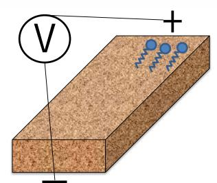
Electrochemical soil remediation uses an electric field and the negatively charged characteristics of PFAS to separate them from the bulk soil. The PFAS are expected to migrate to the anode.
