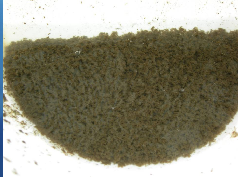
After dosing flocculants
