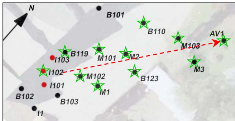
Figure 1. Layout of wells in pilot test area: injection wells (I101, I102, and I103); extraction well (AV1); and performance monitoring wells (stars). Distance between I102 and AV1 is 29.4 m.
