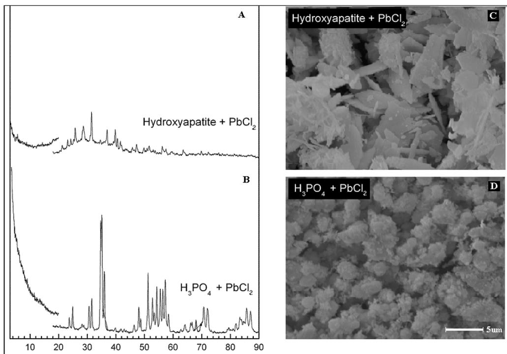
*Figure 6. XRD spectra (A and B), and SEM images (C and D) for the reaction products between hydroxyapatite and  $\text{PbCl}_2$  (A and C) and  $\text{H}_3\text{PO}_4$  and  $\text{PbCl}_2$  (B and D).*
