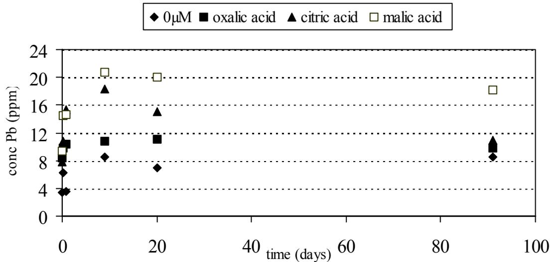
Figure 9. Concentration of Pb in solutions of pyromorphite dissolved in MilliQ-water (0 μM acid) and 40 μM citric-, malic and oxalic acid.
