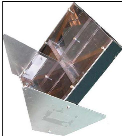
*Figure 1. Rhizotron used for the greenhouse experiment.*
