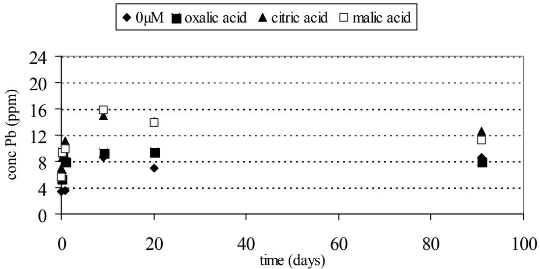
Figure 8. Concentration of Pb in solutions of pyromorphite dissolved in 0  $\mu M$  and 20  $\mu M$  citric-, malic and oxalic acid.
