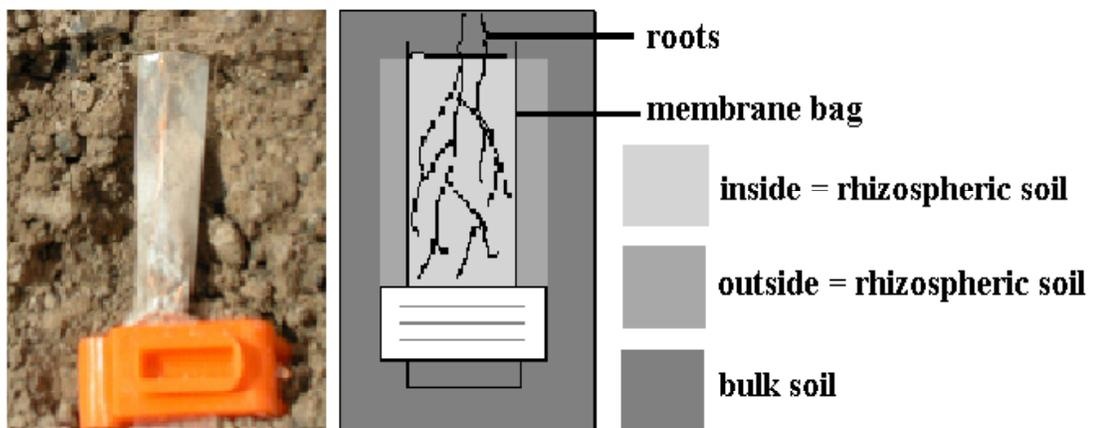
*Figure 3. Dialysis membrane filled with a pyromorphite/soil mixture and roots from Smooth brome grass (left). A schematic picture of the dialysis membrane and its surrounding soil portions (right).*
