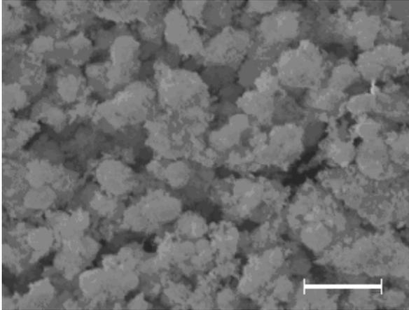
Figure 4. SEM micrographs of pyromorphite crystals. The scale bar represents ca 5  $\mu\text{m}$ . (Source. my own experiments)
