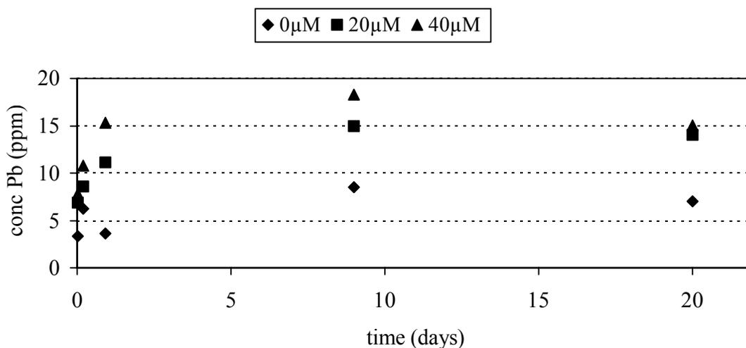
Figure 7. Concentration of Pb in solutions of pyromorphite dissolved in 0, 20 and 40  $\mu\text{M}$  citric acid at different times.
