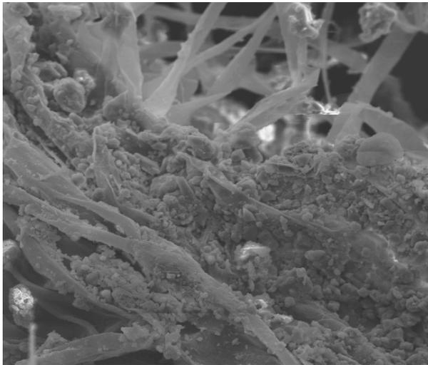
*Figure 10. SEM image of pyromorphite accumulated on the root surface.*
