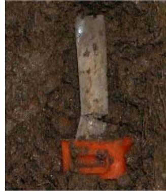
*Figure 11. Broken dialysis membrane.*
