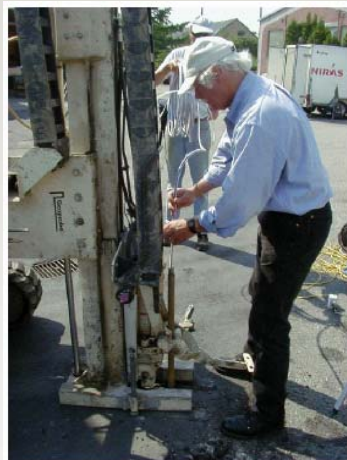
Installation af FLUTe liner i 1,25" GeoProbe rør
